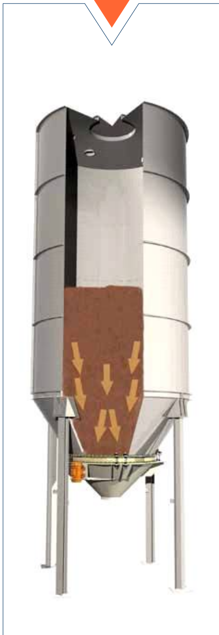
Ratholing Bridging Segregation Incomplete emptying
